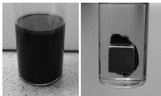
Figure 2. CoNP-TEMPO dispersed in dichloromethane before (left) and after the application of an external neodymium based magnet (right).
